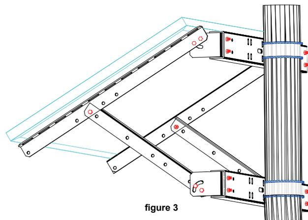
**Step 2.** Gather fixed bracket (C-482A) and align with designated holes along the frame of the PV module for the desired tilt angle. Install one mounting bolt on each side to connect to the PV module frame. Then install the fixed bracket (B-747) along with tilt arm (D-104L/R) to fixed bracket (C-482A). Once done, the bottom portion of mounting kit will be completed.
